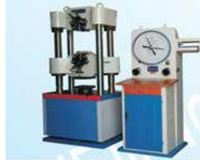
A photograph of a hydraulic universal testing machine. It features a vertical blue frame with a red base. A central vertical column supports a horizontal crosshead. On the right side, there is a control console with a circular dial and various buttons. The machine is designed for materials testing, capable of both tension and compression modes. | 1 | unit |
