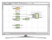
Application configuration allows you to easily create, change or view an IED configuration. The colors of the function blocks relate to the function status in the configuration: unconnected (gray), partially connected (yellow) or fully connected (green).
