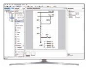
With the graphical display editor, you can easily engineer the single line diagram according to the switchgear arrangement for the IED HMI.
