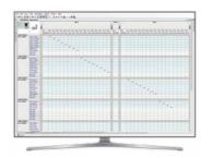
With the signal matrix, you can connect the process termination with any I/O connection point in the configuration in the same way as the traditional trip matrix.
