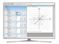
The parameter setting tool allows you to change or view all the parameters that an IED has, for all the setting groups. When reading the parameters from the IED, you can easily compare the values in the PC with the ones in the IED. The graphical representation of protection characteristics supports you in visualizing, for example, distance protection parameter setting.
