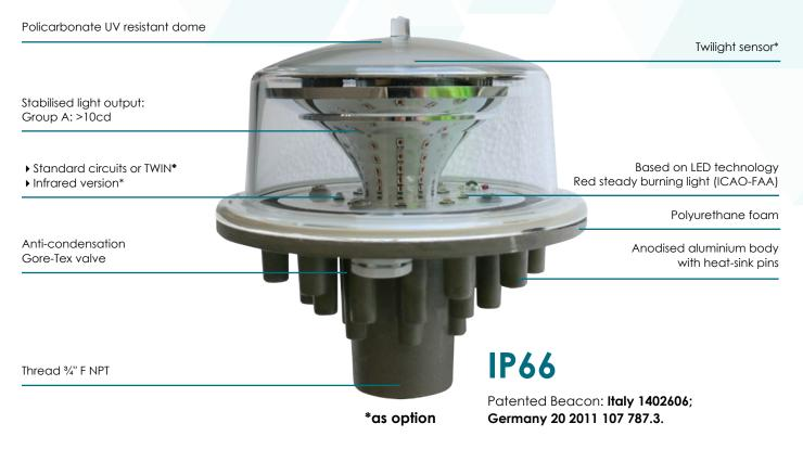
With a low-weight base, designed to dissipate the heat, this LED device is the ideal solution for an **efficient**, **light and compact** obstacle signalling, able to guarantee a **product life exceeding ten years**, along with a **reduced power consumption**.
