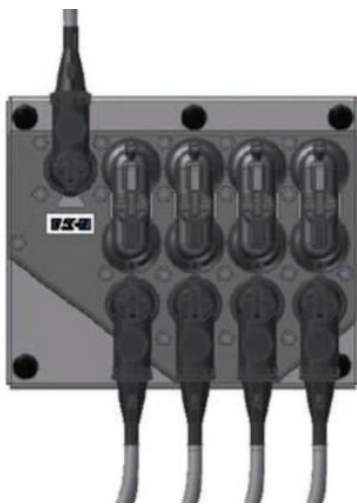
Figure 1 – 600 A source on a 5 way junction bar with (4) 600 A Cleer interfaces and (4) 2 way Cleer and 600 A deadbreak junctions allowing loadbreak switching across a 600 A system.
