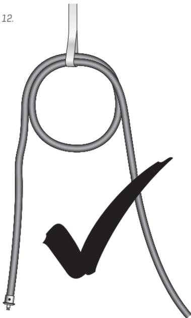
**Correct method of hoisting
