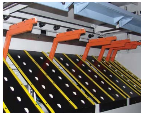
■ Sheet metal being cut can slide with minimum scratch thanks to rollers and bearings on lever type pneumatic sheet metal support system (O)
