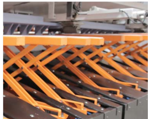
■ X type sheet metal support system operates parallel to ground to support the sheet metal during cutting period (O)
