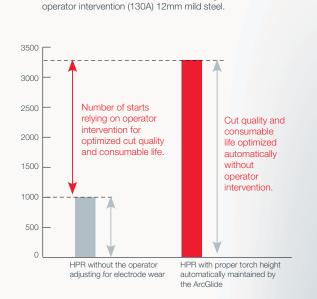
12 mm mild steel number of consumable starts with <0,25 mm deviation from proper cut height without Improper cut height due to not adjusting arc voltage for electrode wear
