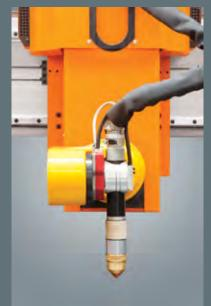
Cutting head moves up and down with Z axis and right and left with X axis.
