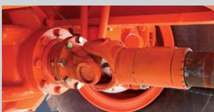
**Transmission Shaft** The use of a reinforced drive shaft and a self-locking nut for the drive shaft's connecting bolt has improved the durability of the drive system.
