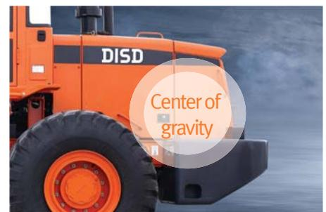
The whole center of gravity has been moved backward, and the real axle load bearing proportion has been increased to 54% , resulting in a tipping load 10% higher than the industry level and greatly improved product stability.
