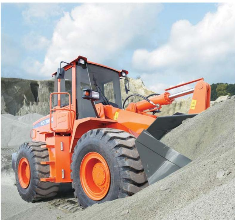
Increasing the tilting angle  $a_3$  in the carry position allows the machine to move on bumpy roads without spilling any material, while increasing the dump angle  $a_2$  enables the machine to dump materials more quickly and completely.
