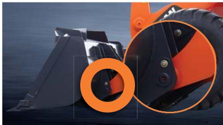
The hinge pins for operating devices in 6 positions have a radius of 5-10mm larger than similar products in the industry. The pin roll sets are made of highly wear-resistant materials and processed with a special heat treatment technology, thus offering greater durability and second-hand residual value.
