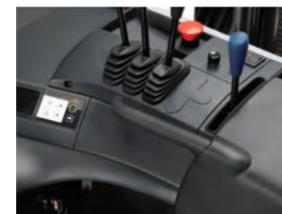
The steering wheel and the levers are oriented to ensure the comfortable posture during operation.
