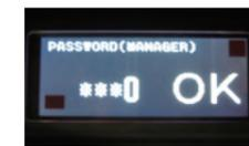
For security to prevent misuses of trucks by unauthorized operators, FRB-9 Series is equipped with this new system, whereby operators have to input their individual code numbers to release the lock before start up the truck.
