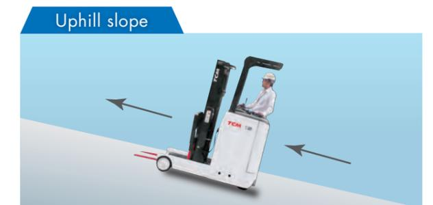
Maintains speed of about 1 km/h if you release the brakes with the accelerator off ("Anti-rollback" feature).
