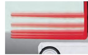
The mast incorporates a soft landing mechanism that reduces the lowering speed just before the forks contact the ground. This greatly minimizes the shock and impact noise (when unladen).
