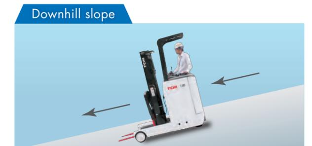
Maintains a constant safe speed (by suppressing acceleration on slope descent). (Travel backward when laden.)
