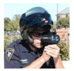
The Stalker XS is the smallest and lightest LIDAR in the Industry, with fast target acquisition and advanced tracking for close-in urban settings.
