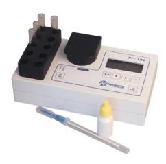
The Pi-102 is a multifunctional, tabletop luminometer that utilizes photomultiplier tube technology. The system features a single read chamber designed to work with both cuvettes and all-in-one collection devices by utilizing an interchangeable extension tower. Able to detect down to 1x10-18 moles of ATP, the Pi-102 is ideal for companies who need to run bioluminescence or chemiluminescence assays and research applications in a laboratory setting.
