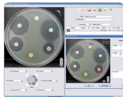
Precision of inhibition zone radius measurement from paper discs : 0.3 mm
