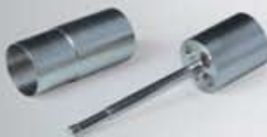
Transdermal Cylinder (Rotating) (USP 6)
