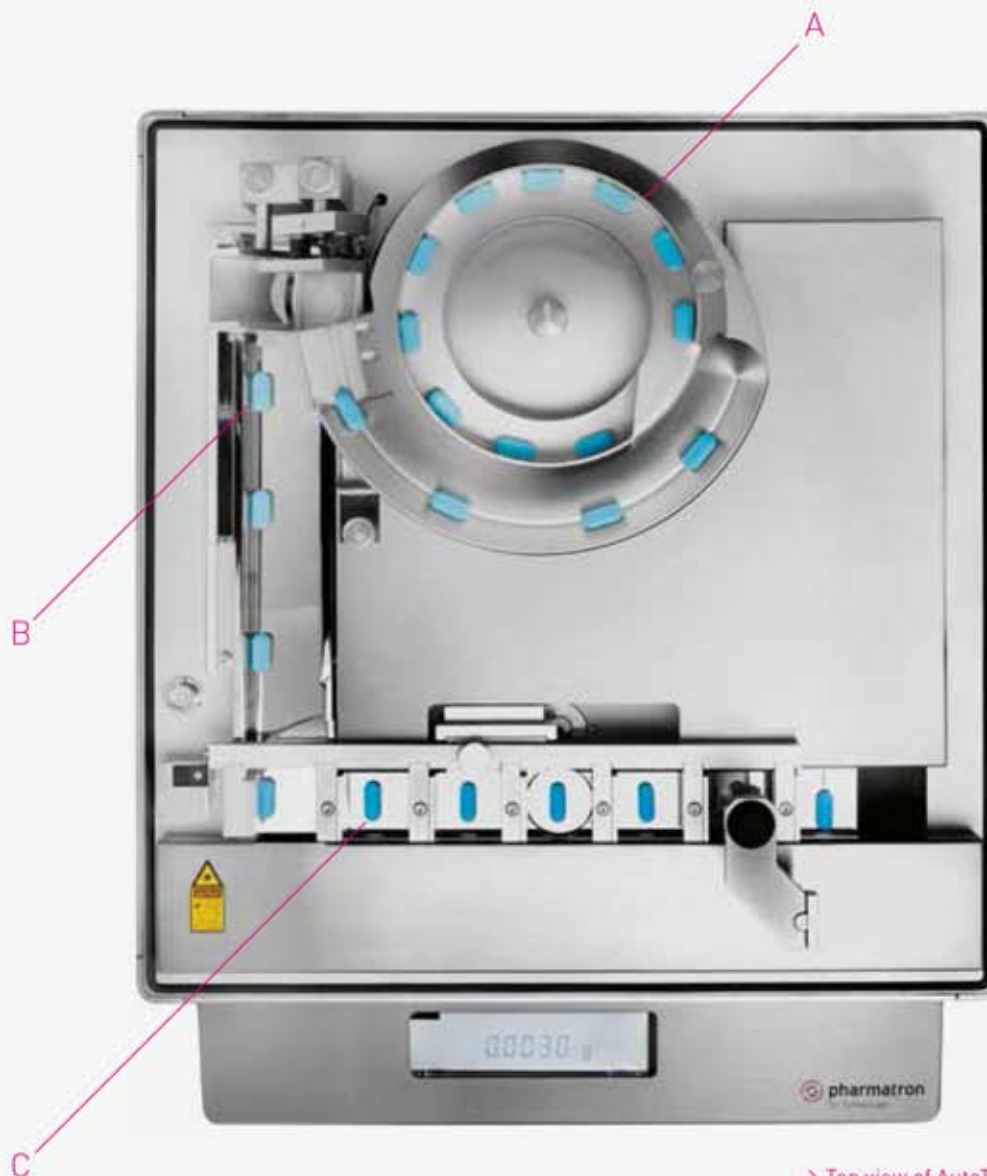
→ Top view of AutoTest 4 A: Vibratory bowl feeder B: Linear feed track C: SmartRake™ and measuring stations
