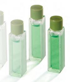
A cost-effective Green Dye standard is available to verify both photometric accuracy and wavelength accuracy of the GENESYS 10S series instruments. With certified values at 260, 430, and 630 nm, this standard provides a check of wavelength and photometric accuracy from the UV to the near-IR.
