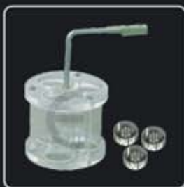
Bolus basket with 3 tubes and guided discs
