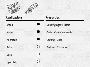
Advantages: Special type for portable belt sanders - For universal use on wood, metal, paint and varnish - Large availability of sizes for all standard machines
