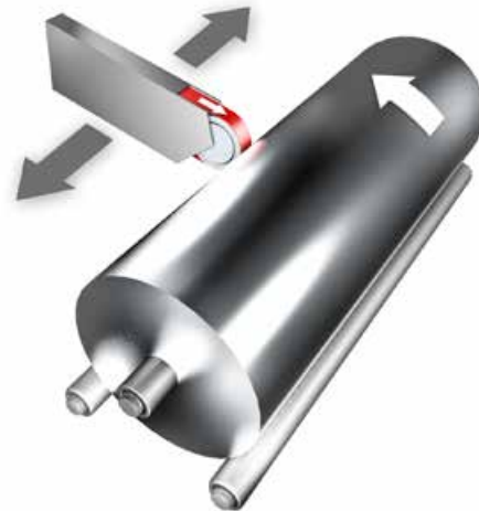
Cylindrical grinding of rollers during roller pass
