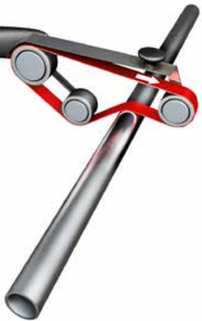
Local grinding of tubes and bars hand-held machines
