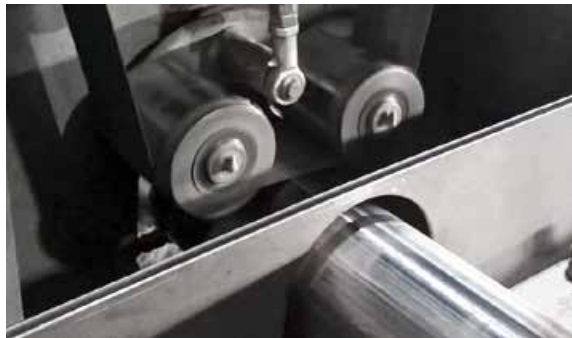
Grinding of longitudinally welded tubes
