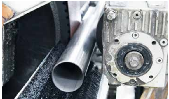
Centerless grinding of tubes and bars
