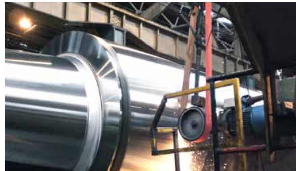
Cylindrical grinding of rollers during roller pass
