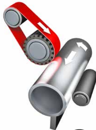
Centerless grinding of tubes and bars
