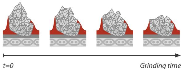
**VSM CERAMICS Plus** grains feature an improved self-sharpening effect when machining high-alloyed steels and super alloys, which are materials that require high contact pressure.
