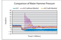
From the above comparison table, the water hammer pressure with Mooha installation is 1.5 times of the water pressure before shielding with the ball valve, and 4.3 times in case of without Mooha installation. So the water hammer difference between with and without Mooha is about 68% attenuated. In addition, according to the long period of the water hammer waveform, the relaxation of the pressure and the shock force due to water hammer could be confirmed.
