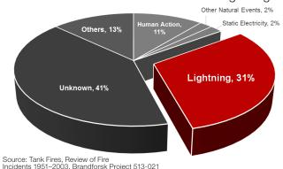
Floating Roof Tanks are especially vulnerable to direct and indirect effects of lightning.
