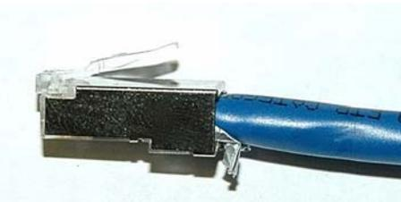
4. Set the RJ45 connector into the housing such that the snap handle is in the notch.
