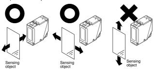
Do not make the sensor detect an object in this direction because it may cause unstable operation.
