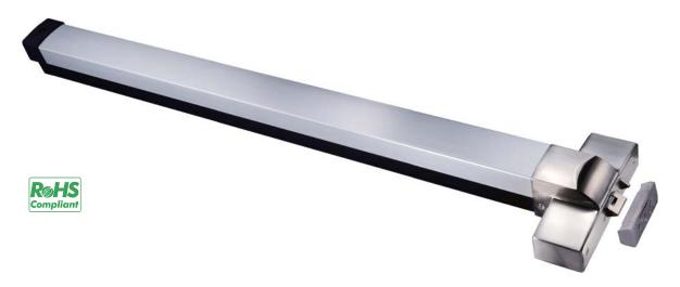
The PBH-350 Series Electromechanical Push Bar is designed for use on emergency exit doors. It provides a convenient means of escape by simply pushing on a horizontal bar fitted across the width of a door. It also features preload release capability that overcomes door preload problems, such as air-conditioning pressure, changes in the weather, warped doors or doors with weather stripping.
