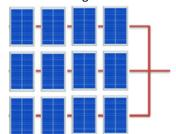
$$\begin{split} &V_{total} = V_{string1} = V_{string2} = V_{string3} = V_{string4} ... \\ &I_{total} = I_{string1} + I_{string2} + I_{string3} + I_{string4} \end{split}$$
