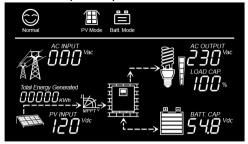
The larger the PV power, the less consumption from battery and therefore the longer backup time.
