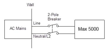
**CAUTION:** Since the inverter doesn't have an automatic protection device against back feed current, it's recommended to install an external AC contactor (see the diagram below). A warning label shall be attached on such AC contractor to remind the user to disconnect the inverter before accessing the circuit.
