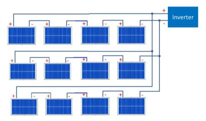
(5) Check again the V<sub>oc</sub> and I<sub>sc</sub> of PV string,
