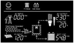
As long as the PV power persists, the load can be powered continuously without consuming power from battery.
