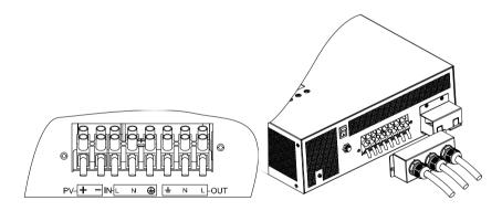
**Step 4** - Fix the AC cover with two screws. Fasten the clamps on the AC cable (not the individual wires) so that the cable won't be pulled off easily.
