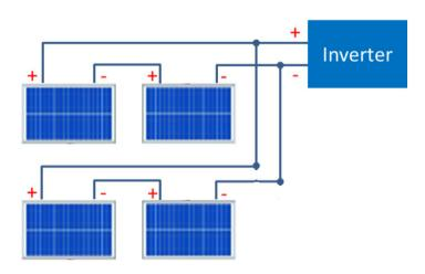
(5) Check again the V<sub>oc</sub> and I<sub>sc</sub> of PV string,
