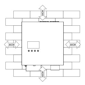
Use 2 screws to mount the inverter to a solid surface. The recommended screw size is  $M5*50\sim65$ mm.
