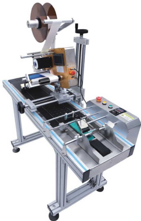
FH-TF200 全自动分页贴标机 AUTOMATIC PAGING AND LABELING MACHINE
