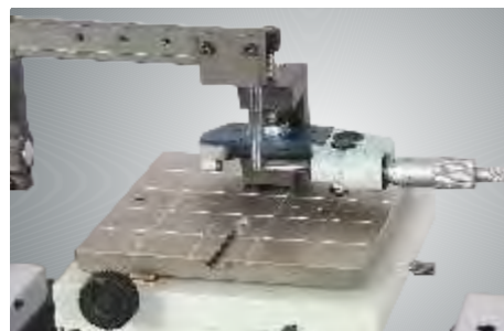
External Micrometer (Below 150 mm) Calibration : Hold on table by using C clamp and measurement by using universal measuring arm
