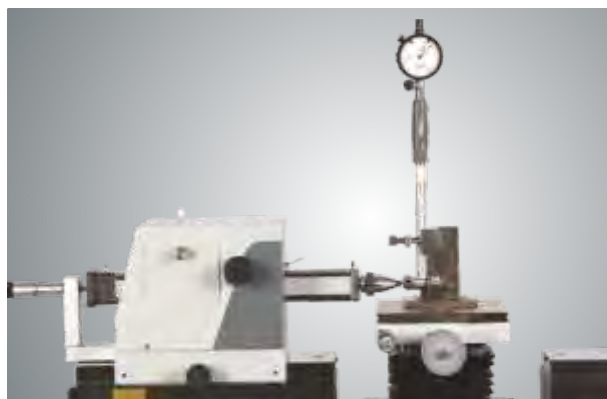
Bore Gauge Calibration : Hold on table by using holding attachment and machine spindle drive unit.
