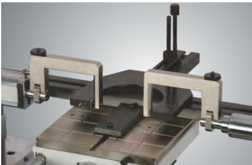
Snap Gauge (below 300 mm) measurement : Hold on snap gauge holding attachment
