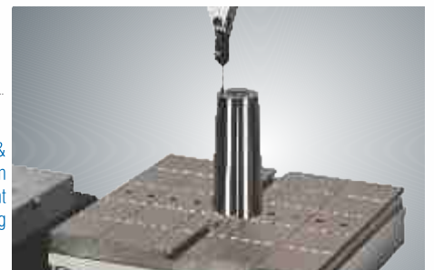
Taper Plug gauge measurement : Using a Single Ruby Ball Stylus with bi-directional probing system of single arm measuring attachment
