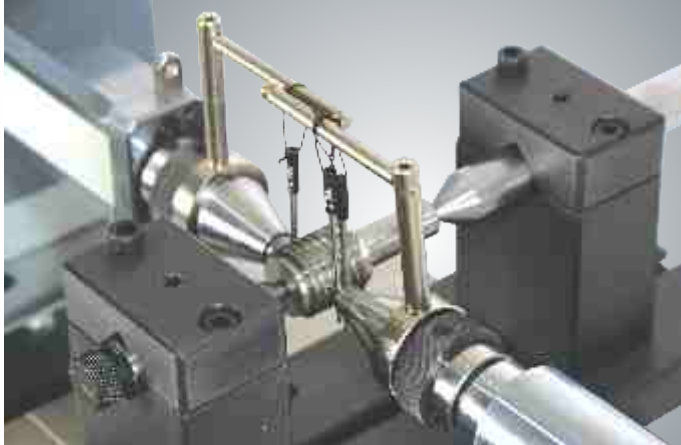
Cy. Thread Plug Gauge (below 100 mm) measurement : Hold between center table
