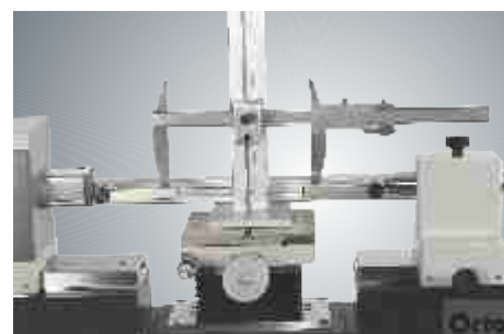
Caliper Calibration : Hold on universal holder
