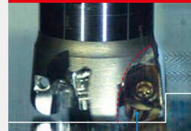
良好に排出されている切りくず Cutting chips which were discharged well
