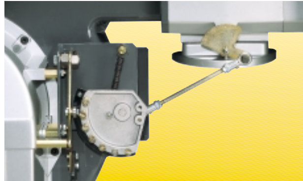
Example of the variable profile cam on RS 70-100-130 burners.
