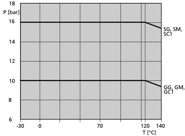
In-service pressure limits and temperature limits as a function of material variant<sup>13)</sup>
