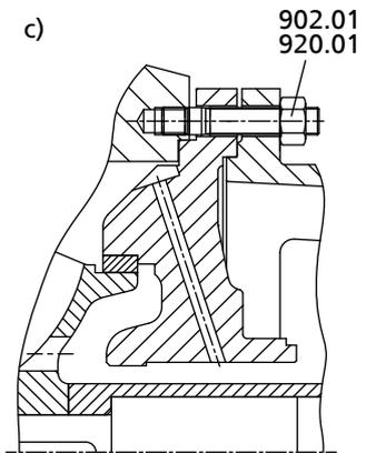
a) Etanorm-R (single-entry) b) Etanorm-R (double-entry) c) clamped casing cover<sup>20)</sup>
