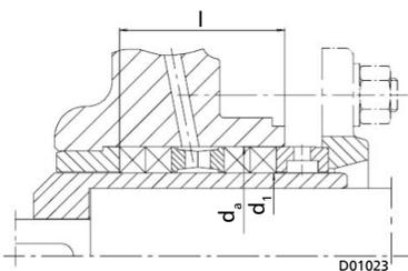
Dimensions of the gland packing chamber
