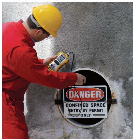
Confined space testing with the MultiRAE Lite
