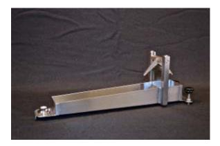
The <u>**"Bostwick"**</u> is a long trough with 0.5 cm graduations along the bottom. The trough is separated near one end by a spring-loaded gate. This forms a chamber where the sample is loaded.
