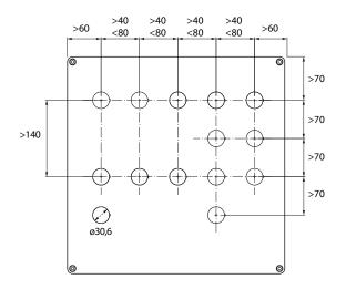
The installation of Ex operators and instruments inside the enclosures can be done according to the limits of certification in terms of distance and heat dissipation.
