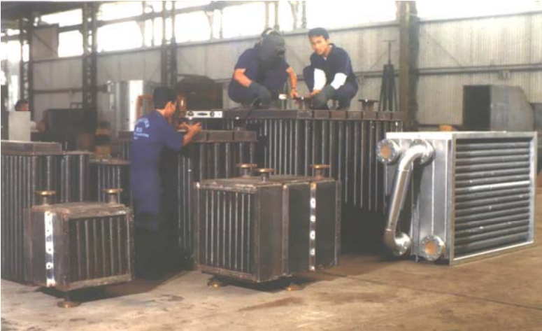
Thermal Oil to Air for Air Heater
