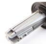
The rollers over the circumference of the mandrel allow to achieve a perfect surface of the hole.
