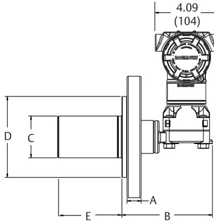
**Diaphragm assembly and mounting flange**
