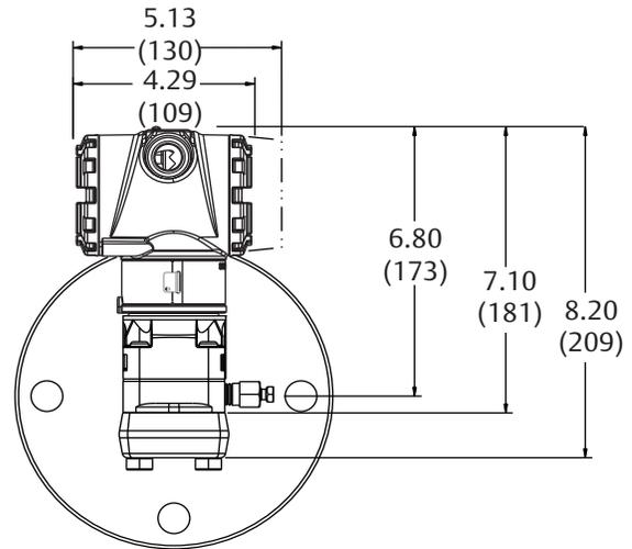
**Optional flushing connection ring (lower housing)**
