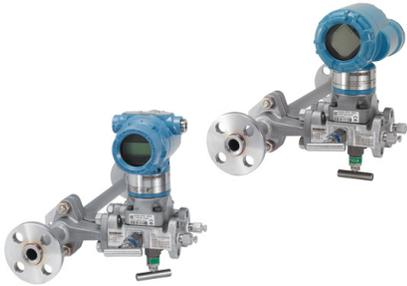
Rosemount 3051CFP Integral Orifice Flowmeters enable highly accurate flow measurement in small line sizes. Integral Orifice utilize precision honed pipe section for increased accuracy and self-centering plate design to prevent alignment errors that magnify measurement inaccuracies in small line sizes.
