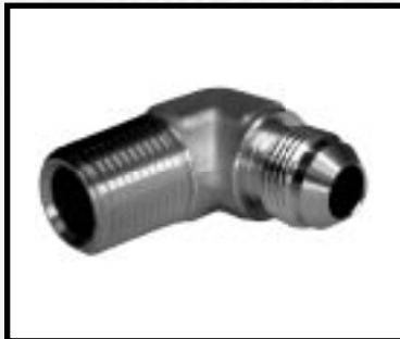
Male JIC 37° x Male NPT 90° Elbow (Stainless Steel)
