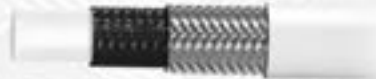
SFT-Si SuperFlex™ – Teflon® PTFE smooth liner, fiberglass braid, SS braid, and silicone cover.
