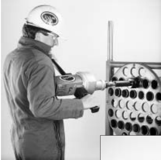
The 22488 Electric Rolling Motor rolls tubes up to 3" OD.
