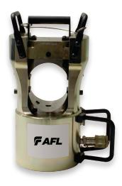
The 100A Single or Double Acting Press is designed for the installation of compression fittings. The 100A develops 100 tons of force at 10,000 PSI. A special piston facilitates operation in single or double acting mode. Redesigned for portability, the press now weighs 95 pounds.
