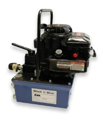
The 15GBM is a gas powered pump that produces 10,000 PSI of hydraulic pressure. It is designed to handle any high pressure tool up to and including the 60 ton press. The two-stage pumping system allows for rapid ram advance. The "suc-o-matic" valve helps tools retract faster. The manual control has three settings: advance, hold and retract. Whether making one crimp or 1,000 crimps, the 15GBM is the lightweight, portable answer.
