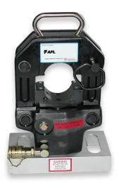
The 60-Ton Single or Double-Acting Press is unsurpassed in the industry. The compression tool develops 60 tons of force at 10,000 PSI for the installation of electrical compression fittings. The major feature of this tool is a double-acting ram head. The result is more positive retraction, which reduces cycle time. A special piston facilitates operation in single or double-acting mode.
