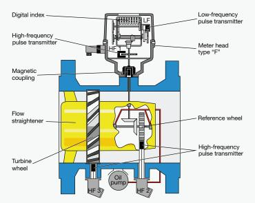
The gas flow is constricted to a definite cross-section and drives a coaxially mounted turbine wheel. The speed of the turbine wheel, which is proportional to the flow rate, is reduced by gearing and transmitted to the mechanical digital index.
