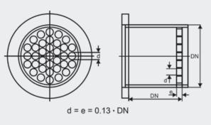
LP-35 Perforated-plate Straightener
