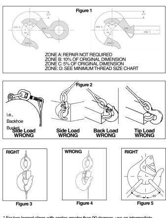
\* For two legged slings with angles greater than 90 degrees, use an intermediate Ink such as a master link or bolt type shack the to collect the legs of the slings. The intermediate link can be placed over the hook to provide an in-line load on the hook. This approach must also be used when using slings with three or more legs.
