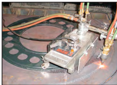
Circle Track Part # BCD19109 Cuts 1 1/2 - 14" (40 - 360mm) inside and 30 - 45" (770 - 1,150mm) outside, counter weight recommended.
