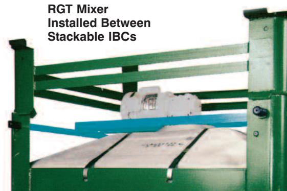
RGT Mixer Installed Between Stackable IBCs
