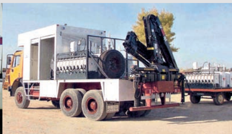
Lube truck , 502 Series hose reel , PM4 oil pumps and PM3+3 grease pumps.
