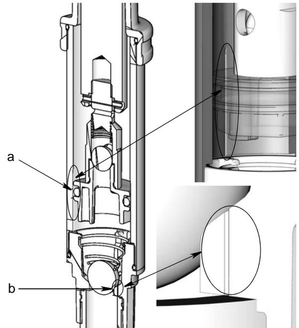
**FIG. 4** a = Pump cylinder relief passage
