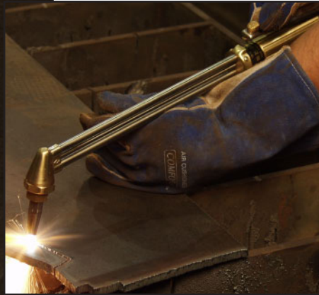
Model MK-300 shown cutting with 75° head
