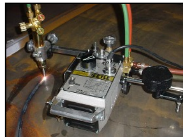
Circle Cutting Bar Set option cuts circles from 1½ - 96 in (38-2450mm) diameter. Part#ZS31858
