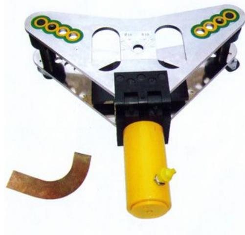
**Horizontal and Erective CB-125D Flat Bender** bending two kinds of legislative functions, aluminum, copper width 40,50,60,80,100,125 mm thickness 4,5,6,8,10,12.5 mm;
