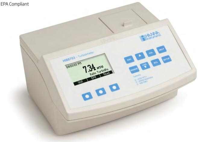
The HI88703 Precision Turbidity Benchtop Meter is specially designed for water quality measurements, providing reliable and accurate readings, especially in the low turbidity range. The instrument is based on a state-of-the-art optical system which guarantees accurate results, assures long term stability, and minimizes stray
